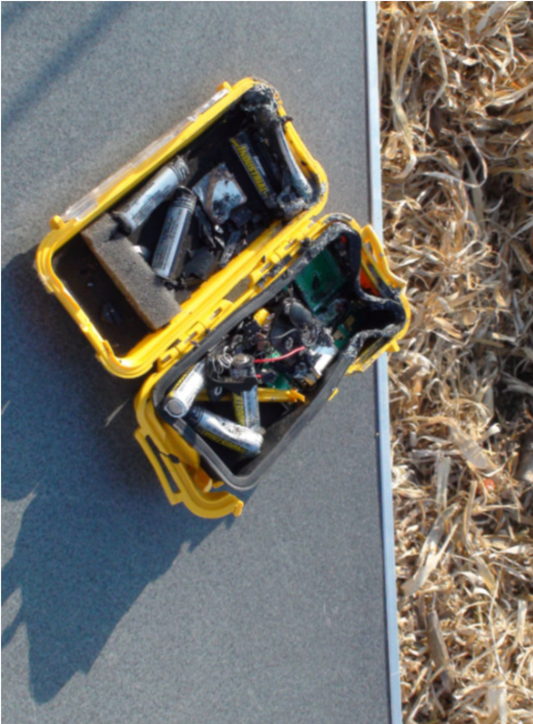
An MT-AIO, carried as rocket payload, after auguring in from 12000 feet.
